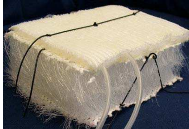
Fig. 2: Possible arrangement of the sensor fibres and the fluidic actuator tubes
