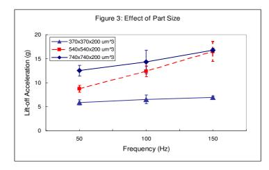
Figure 3 shows the experimental results. As the part size decreases the liftoff acceleration also de-creases despite the decreased mass. This result indicates that the surface area related forces dominate the motion of the parts. The lift-off acceleration increases with
