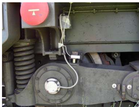
Fig. 6 The position of the acceleration on the housing of the axial bearing
