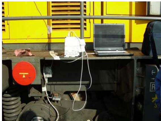
Fig. 4 The measuring place with the acceleration sensor, the central appliance EUROACC and a laptop computer
