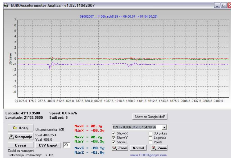
Fig. 7 The appearance of the user interface at the moment when the locomotive went down from a turntable at the railway station “Niš”
