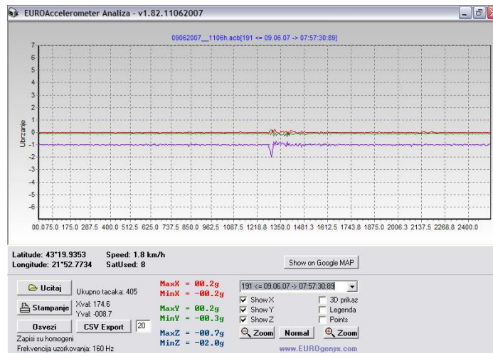
Fig. 8 The appearance of the user interface at the moment when the locomotive crossed over the turnout 1
