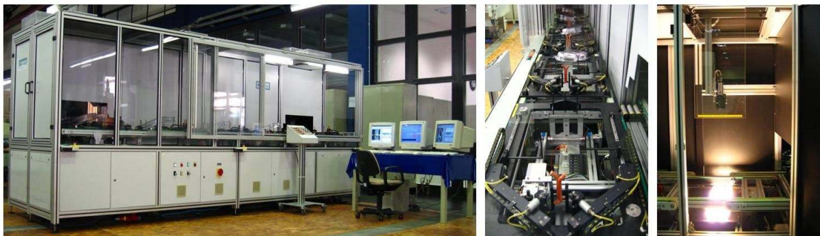
Figure 4. Automated system for the inspection of automobile headlight glasses (left). Headlight glasses mounted on pallets fed by conveyor belts (middle). Internal modular machine vision stations (right).
