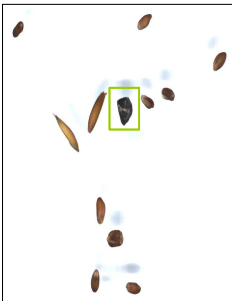
Figure 1: Online volume flow of the cereal sample in free fall under incident and transmitted light Figure 2: selected single kernel images
