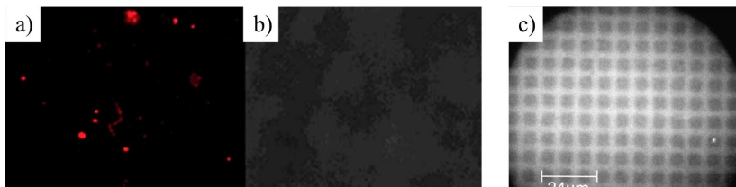
Fig. 6.12: a) Fluorescent image of randomly biotinylated probes on a chemically treated GaN surface and b) of a non-biotinylated surface for comparison [120]. c) Fluorescent image of Alexa Fluor 488 penicillinase conjugates selectively immobilized on a patterned (pattern size 4 \times 4 \mu\text{m}^2 ) functionalized GaN [158].
