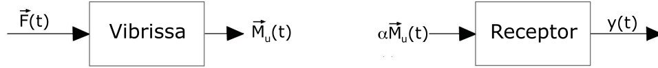
Fig. 6. Model of the stimulus transmission from the vibrissa to the mechanoreceptors. \vec{F}(t) - input signal (disturbing force), \vec{M}_u(t) - control torque, \alpha - dimensional factor, y(t) - output signal, [24].
