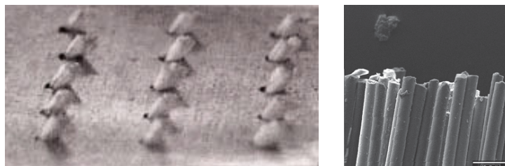
Fig. 16. left: Tuft with prespecified pitch angle; right: Microscope image of a tuft, [11]
