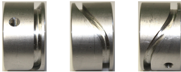
Fig. 35. Cam drum in different views; left: dwell phase; middle & right: movement phase, [29]
