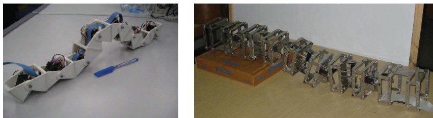
Fig. 9. left: Prototype Cube, [19]; right: Mobile Robot with Worm-like Movement, [20]
