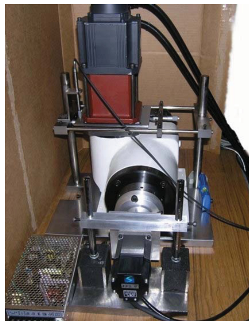
Figure 8. Rotary axis and measurement components
