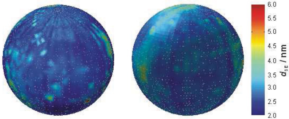
Fig. 8. Topographic maps of the surface layer thickness measured by spectral ellipsometry (not calibrated). Left AVO28-S5, right AVO28-S8. The rainbow colour code ranges from 2.0 nm (blue) to 4.5 nm (yellow).
