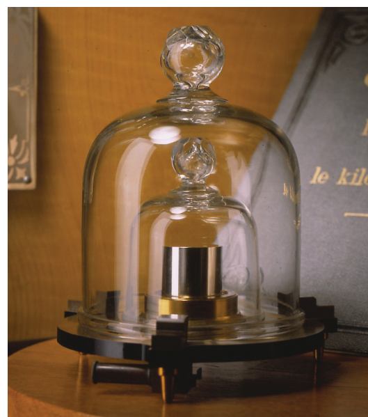
Fig. 1. The Swiss official kilogram (prototype No 38).
