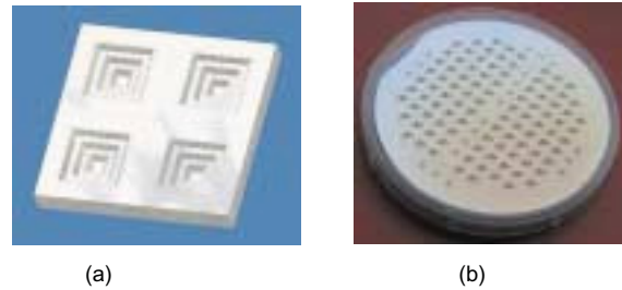
Fig. 16 Layout of the 3D test artifact for micro/nano CMMs is shown in (a), and a photo of a wafer of such artefacts fabricated using photolithography based micromachining techniques is shown in (b) [11].
