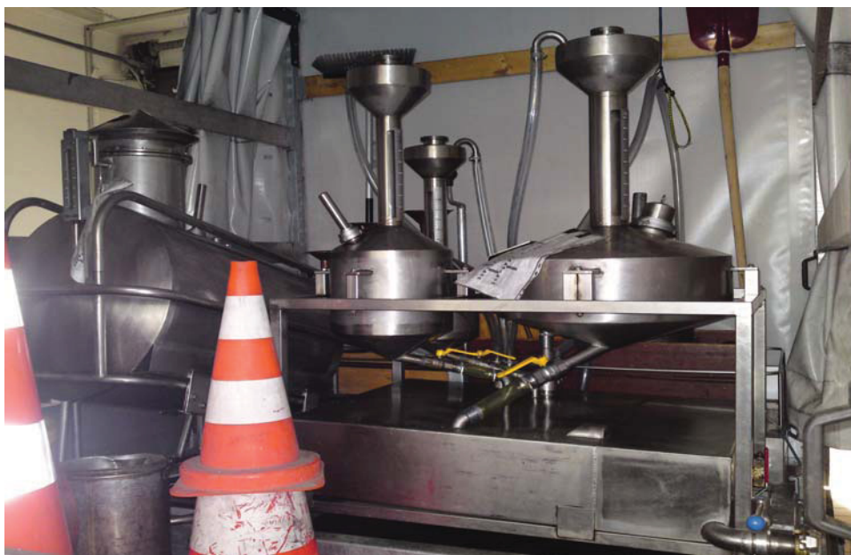
Fig. 2 set of gauging tanks and additional tanks at the bottom, property of the Thuringian State Authority of Metrology and Verification
