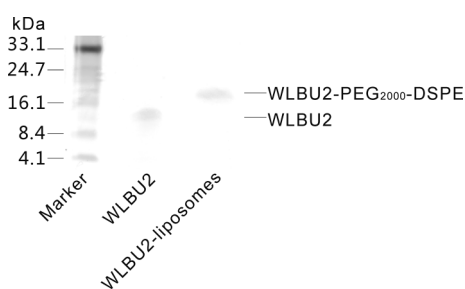
Fig. 2 Detection of the conjugation of WLBU2 with NHS-PEG 2000 -DSPE in WLBU2-liposomes using SDS-PAGE.
