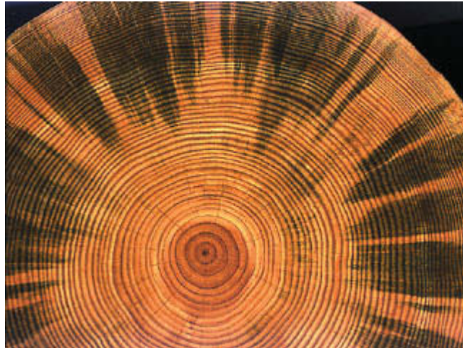
Figure 1.1: Cross section of Norway spruce sapwood infected by the blue stain fungus C. polonica . Photo: E. Christiansen.
