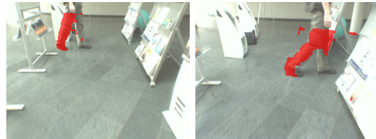
Fig. 5. Detection of a moving person that is walking from left to right while the robot is moving forward. Image regions, where motion was detected, are highlighted in red. Our approach correctly detected the motion of the leg that is moving forward, while the leg that stands on the floor is classified as static.
