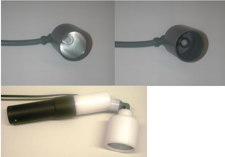
Fig. 7: Optimized optical sensor with reflector shield (left: with inner reflection layer, right: without inner reflection layer, below: construction for sticking in prepared holders in switchboards)
