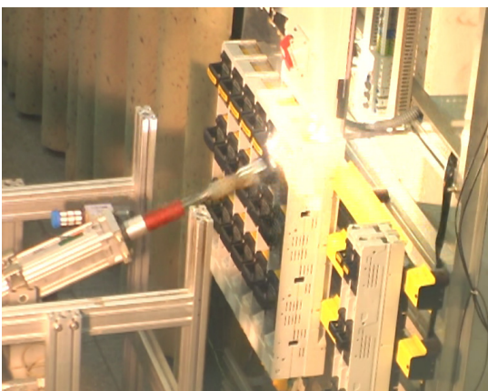
Fig. 12: Fuse withdrawing test No. 19 (according to Tab.6) with oszillogram
