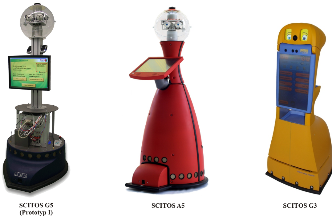
Figure 1.2: Robot systems used in the SerRoKon and CompanionAble projects: Prototype of the research platform SCITOS G5 developed within the project, shopping robot SCITOS A5 used for field tests, and SCITOS G3 developed for home environments.
