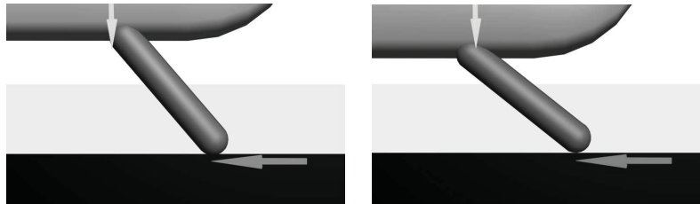
Figure 3: Locomotion of the robot due to the friction force
