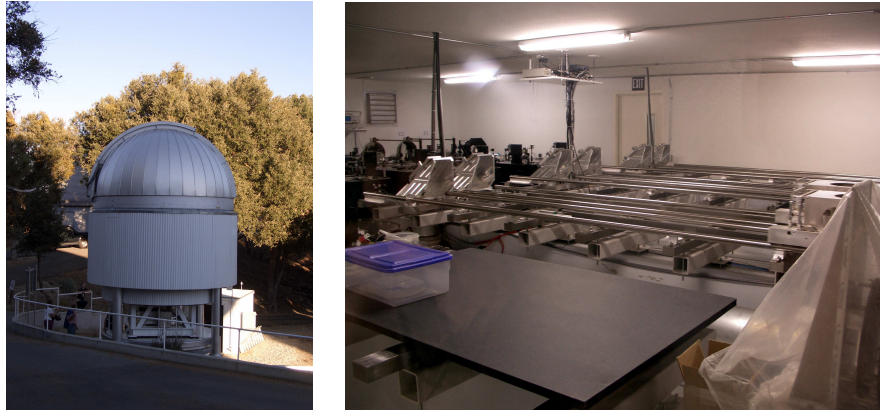
Figure 2.7: One of the 1 m telescope of the CHARA array (left) and part of the delay lines under the CHARA laboratory (right)
