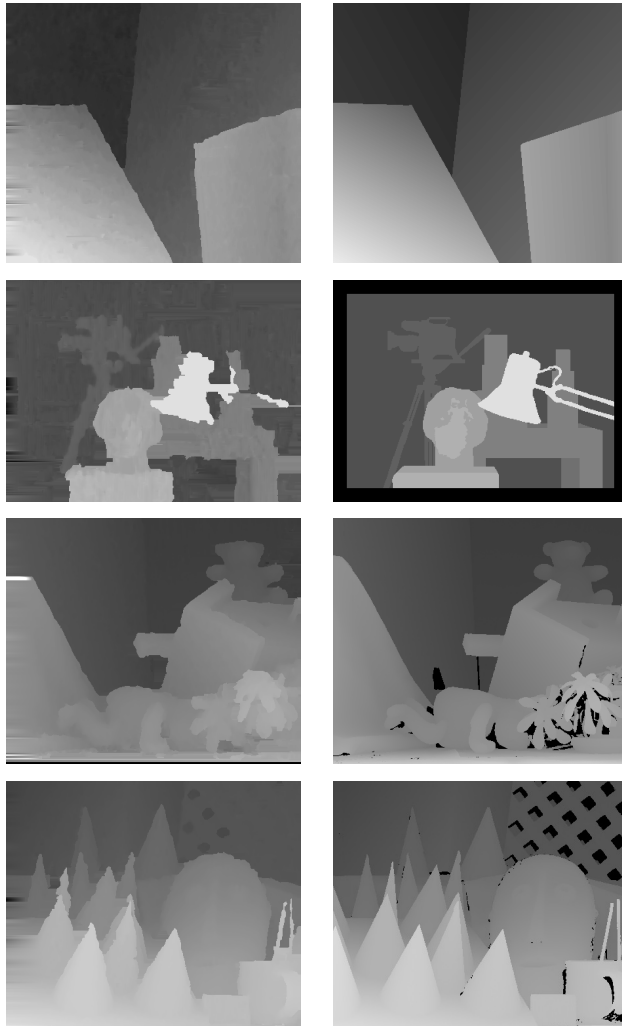
Figure 3.12.: From top to bottom these are disparity maps of the Venus, Tsukuba, Teddy and Cones scene. The first column shows the result of the proposed SNCC for block-matching stereo and the second column the ground truth disparity maps. The disparity values are encoded by means of intensity. Near pixels are bright and far pixels are dark. Black pixels in the ground truth disparity maps indicate unavailable ground truth disparity.
