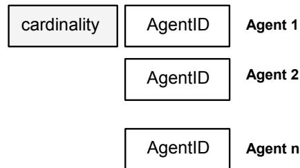
Figure 7.16: Format of the location cache in a normal platform
