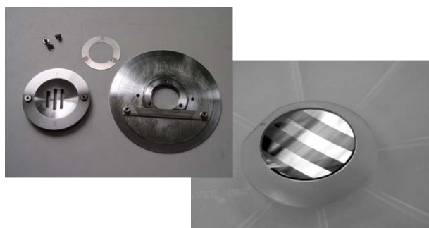
Fig. 3 Etching mask (left), substrate holder (middle) and Al-coated master grating with two different blazed regions arranged in a stripe pattern (right)
