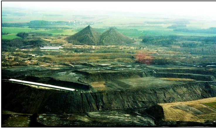
Figure 1: Ronneburg mining area during active mining time. In the front the open pit, in the back the leaching heaps. (in Chem. Erde - Geochem. Vol. 65, 2005)
