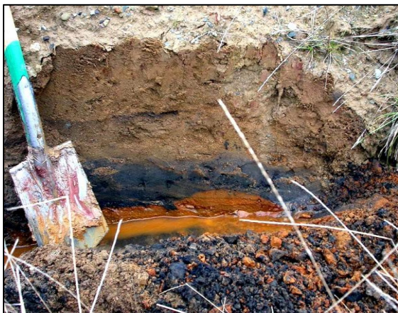
Figure 4: Hardpan layer enriched in Mn, Fe and other metals. This showed a recent mineral layer formation connected to a strong interaction with the groundwater. (in Chem. Erde - Geochem. Vol. 65, 2005)
