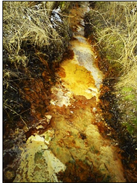
Figure 2: AMD and ron precipitates in the Gessen creek near Gessenwiese [a]; Fe-, Al-, Ni-precipitates near Northern heap [b] (2009, own photo)
