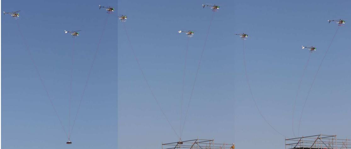
Figure 7.5: Utrera 2009 - Multi-lift configuration: Flight - During deployment - After deployment
