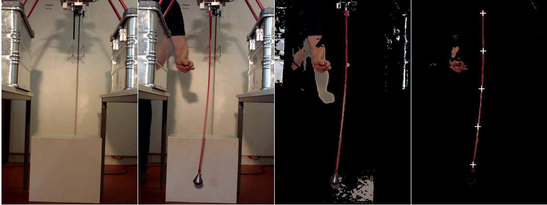
Figure 5.6: Video processing (left to right) - Zero image, experiment image, difference image, processed result
