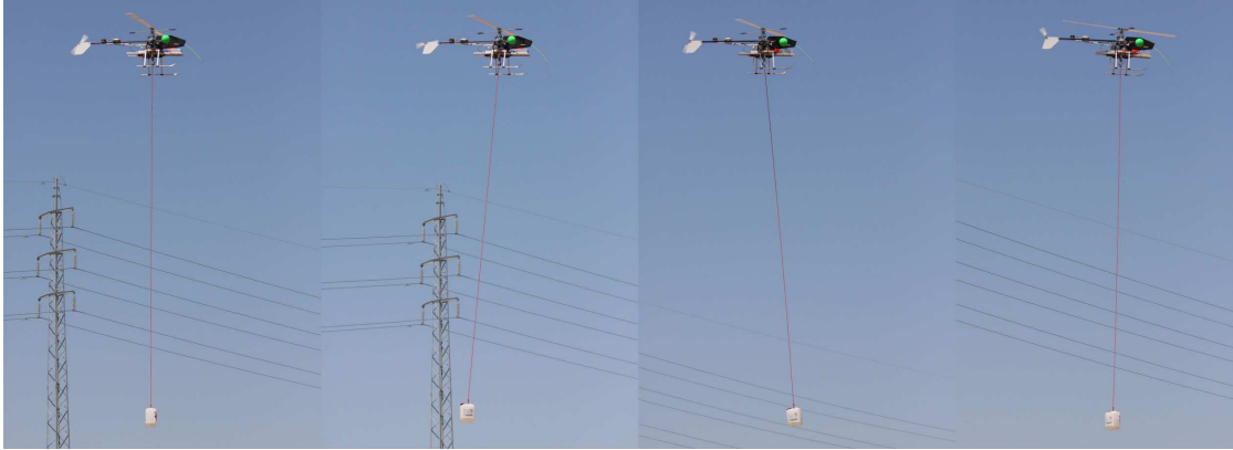
Figure 7.3: Utrera 2009 - Typical slung load motion: Hovering - Acceleration - Deceleration - Hovering
