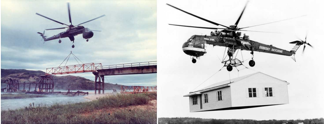
Figure 1.1: Slung load configurations of a CH-54a skycrane (© United States Army - Redstone Arsenal, AL)
