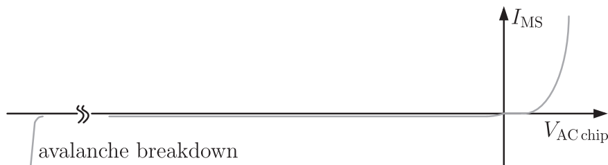
Figure 2.10: Current-voltage characteristics of a SCHOTTKY diode
