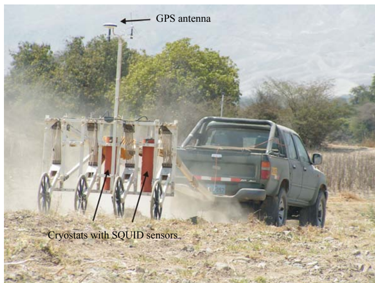
Notes: The vehicle can carry up to three helium cryostats - here a two channel configuration is shown
