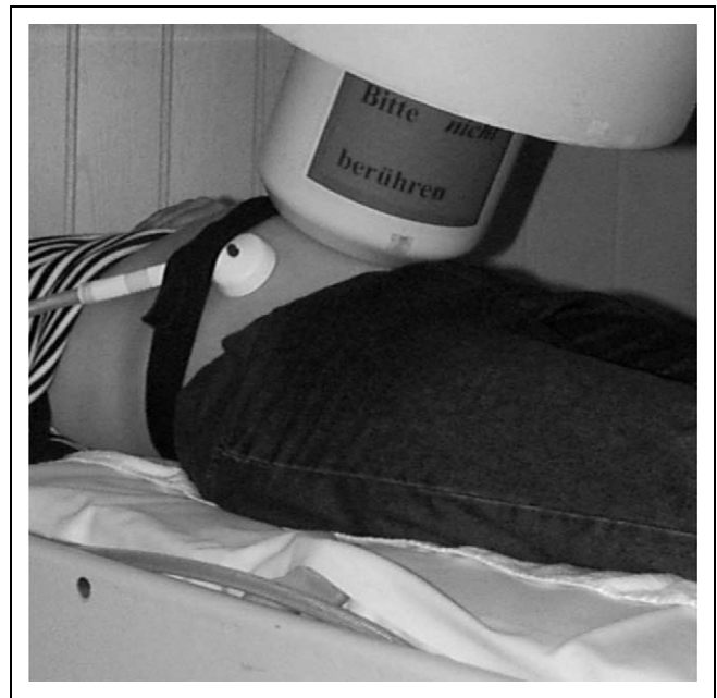
Figure 1. Experimental setting inside the magnetically shielded room with the sound applicator and Dewar in position. The recording system consists of 31 helium-cooled superconducting quantum interference devices (SQUIDs) fed by the corresponding number of symmetrical first-order gradiometers (coil diameter of 20 mm; baseline of 70 mm) arranged in an array of 145 mm in diameter. The system noise is below 10 \text{ fT Hz}^{-1/2} above 1 Hz.
