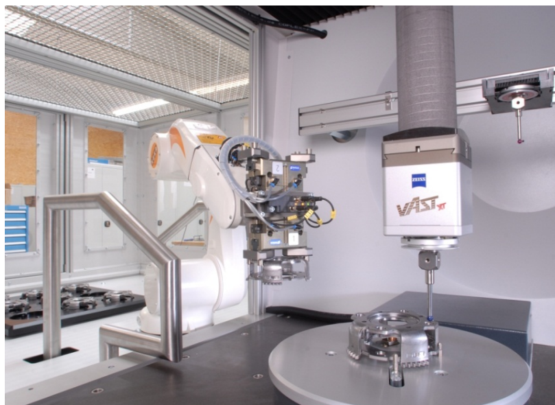
Figure 4: Example for faster metrology due to the automated integration of a coordinate measuring machine into material flow by robot loading.
