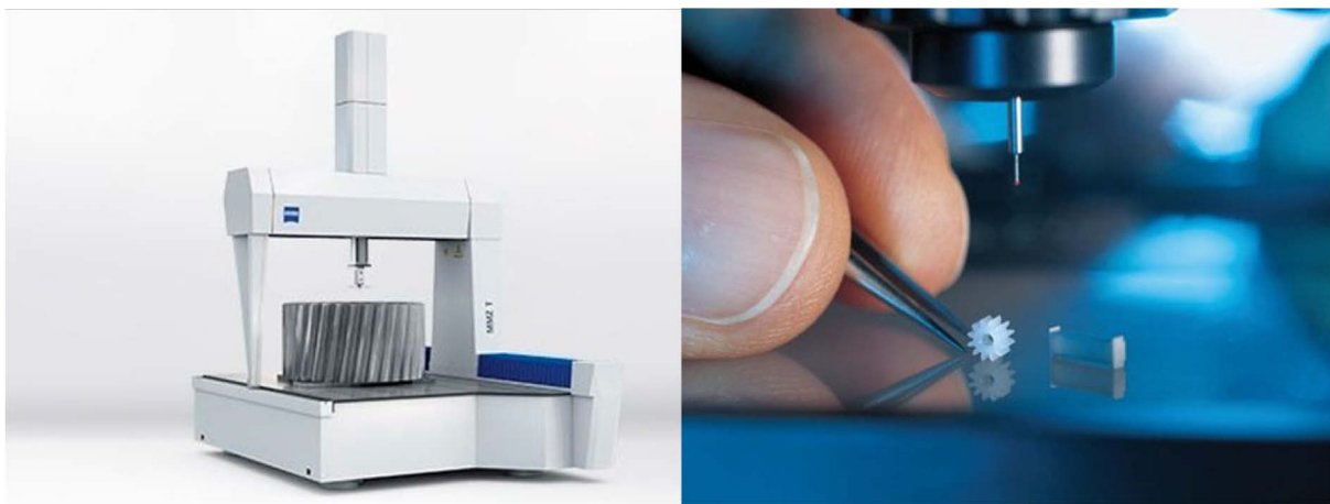
Figure 5: Range of gear metrology with coordinate measuring machines from macro-scale gears for wind energy systems [14] to micro-scale gears for watches [15].
