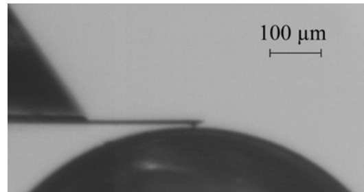
Figure 2- picture of cantilever and load button using the long distance microscope camera
