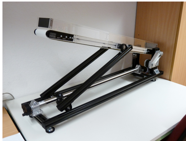
Figure 5: Experimental environment for worm-like locomotion systems [15]
