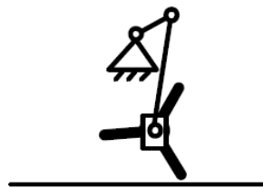
Fig. 1a: Technical principle of the basic mechanism for height adjustment
