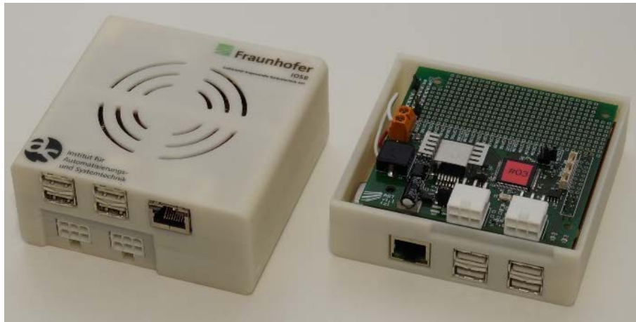
Fig. 4: SAM Boxes. The opened case shows an additional prototyping area.
