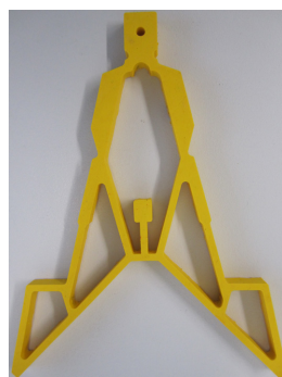
Figure 8. Compliant gripper without sensor elements from [8]
