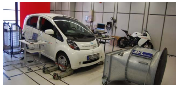
Figure 2.2: EV on a dyno test bench
