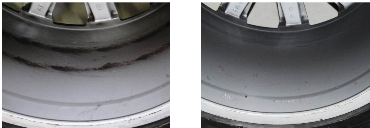
Figure 6: Wheel rim of surface machined disc (left) and standard disc (right)
