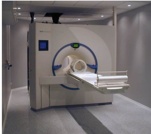
Figure 2.1: Siemens MT-Trio 3T MR scanner (used to acquire the data used in this thesis), Max Planck Institute for Human Cognitive and Brain Sciences.
