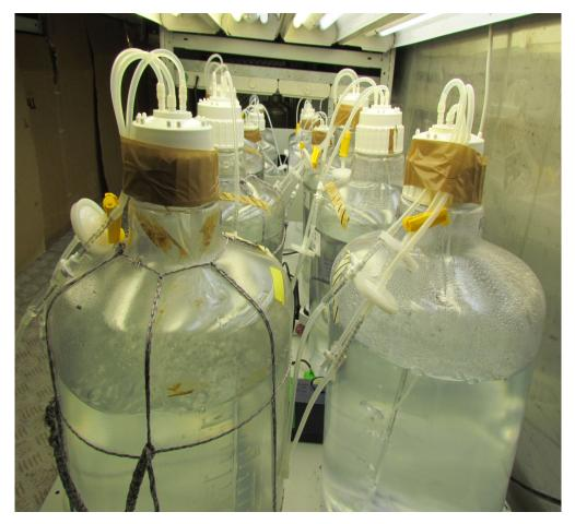
Bioreactor cultures conducted in Jena laboratory using 25L and 10L of *Ulva* culture medium in polycarbonate bottle.
