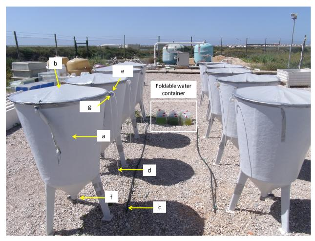
**Figure 45**: Aquaculture set-up of 200 L in (a) cylindrical and conical tanks. (b) Tygon film. (c) Pump. (d) Silicon tubing ( $\emptyset$  int. 2mm ×  $\emptyset$  ext. 4mm 228-0703 VWR). (e) HEPA-Vent ( $\emptyset$  50 mm, Whatman) filters. (f) Inlet of air and outlet of samples. (g) The right direction where the disconnection should be made to get the samples.
