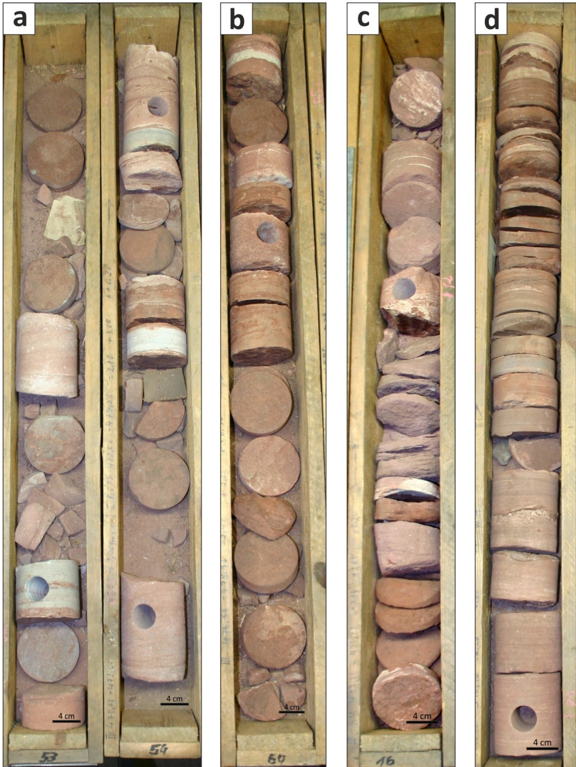
Fig. A 19: Drilling core Fh13, photos: a) sandflat sandstone (sample Fh13-46, Fh13-47, Fh13-50, Detfurth Formation); b) eolian sandstone (sample Fh13-88, Detfurth Formation); c) sandflat sandstone (sample Fh13-12, Hardegsen Formation); d) sandflat sandstone (sample Fh13-85, Volpriehausen Formation).
