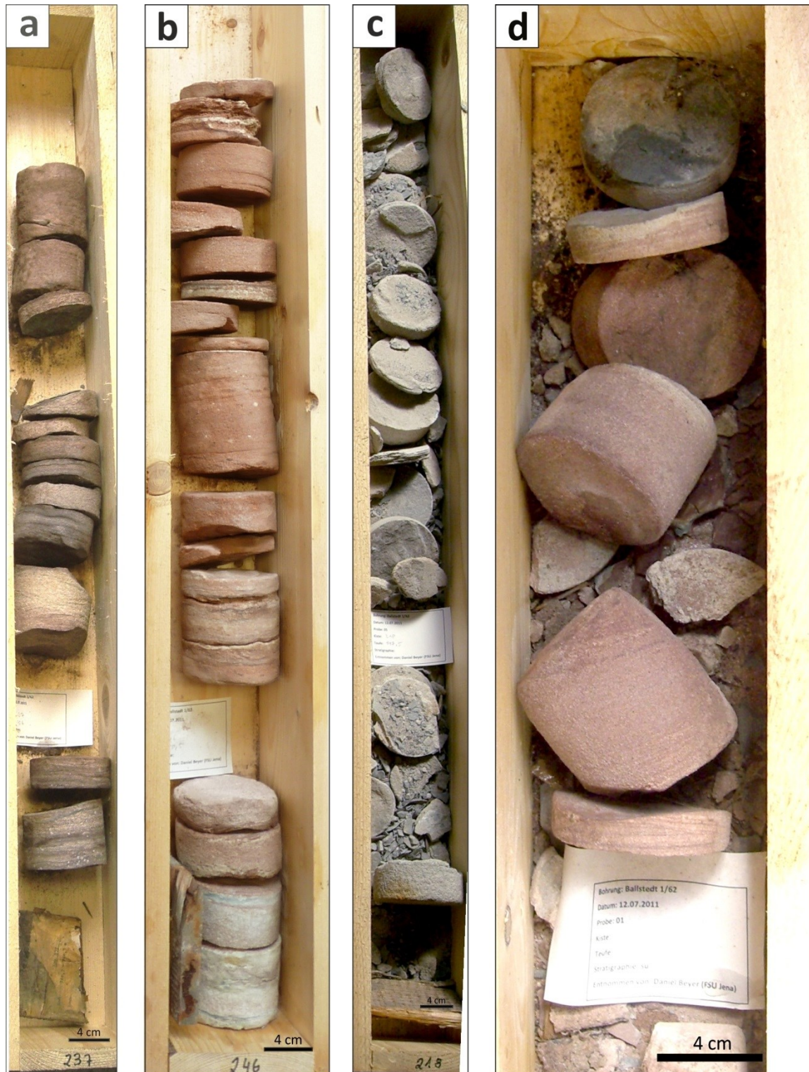
Fig. A 20: Drilling core Ballst, photos: a) lacustrine sandstone (sample Ballst-8, Bernburg Formation); b) lacustrine sandstone (sample Ballst-9, Bernburg Formation); c) sandflat sandstone (sample Ballst-5, Volpriehausen Formation); d) sandflat sandstone (sample Ballst-1, Volpriehausen Formation).
