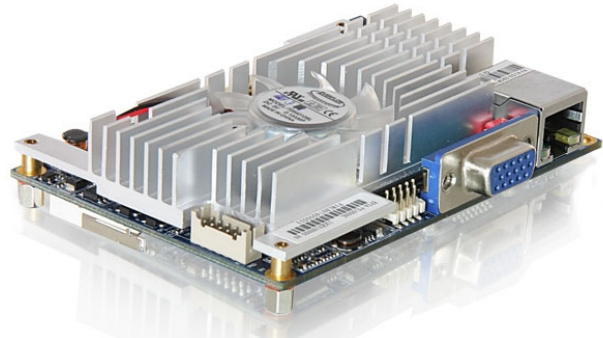
Figure 4. The software add-on: x86-compatible VIA board for all computational-intensive applications [6]
