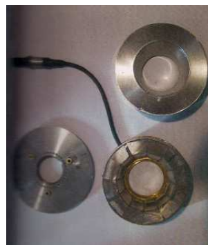
Figure 3.13: Photo of Halbach cylinder magnet system picture. It shows its different; parts housing lower part, housing top and the twelve symmetrically aligned trapezoidal permanent magnets.
