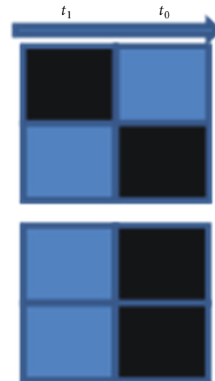
FIGURE 5: Two spatiotemporal stimulation sequences to be provided by the microelectrodes of the 3D MEA.
