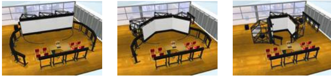
Figure 2.1. Illustration of the CAVE-like immersive virtual environment in the FASP Laboratory at Technische Universität Ilmenau (FASP, 2014)
