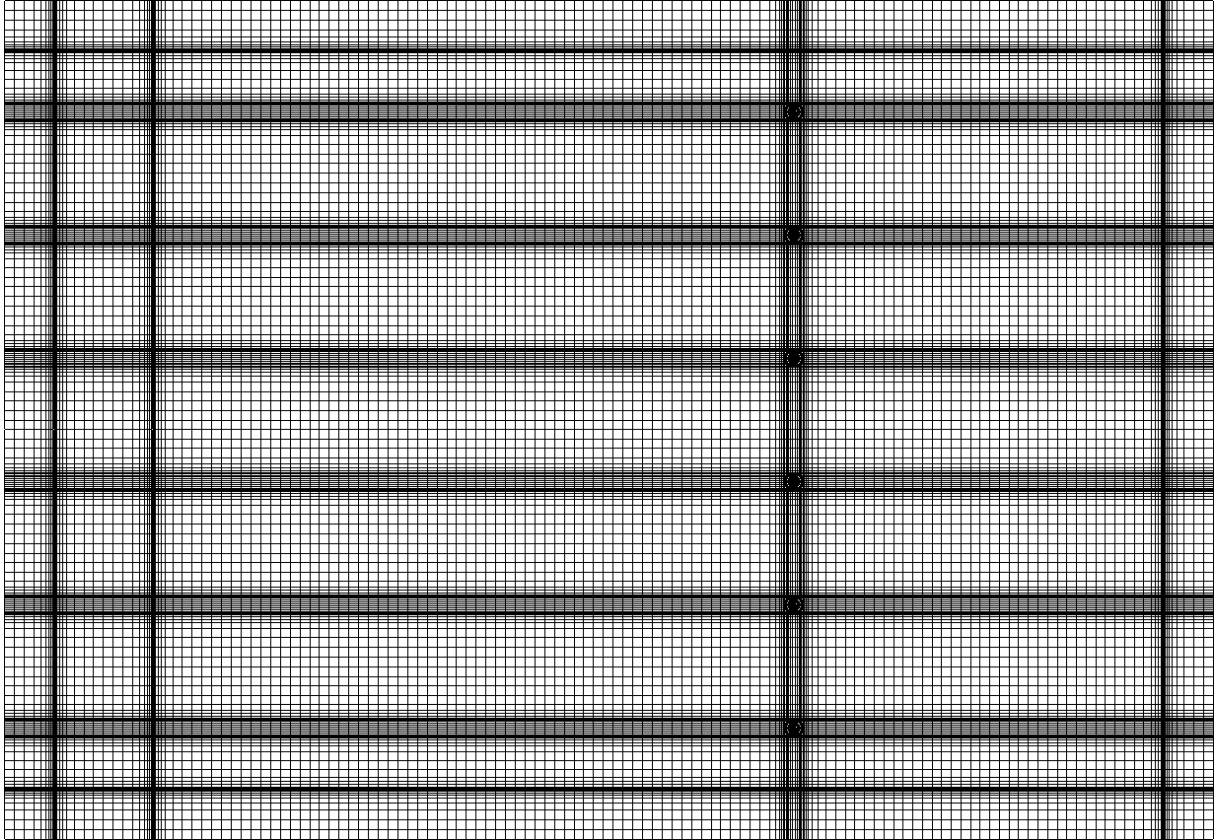
Figure 8.1: Plane view of the top side of the block-structured hexahedral mesh topology, generated using the commercial software ICEM CFD, for the tank simulation. The related geometry is depicted in Figure 6.1.
