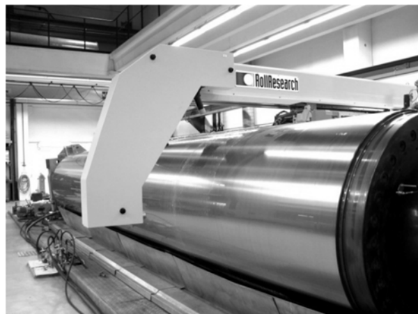
Fig. 1. Four point roll measuring device of a grinding machine. 1
