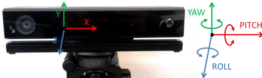
Figure 4. Position and orientation of the camera coordinate system
