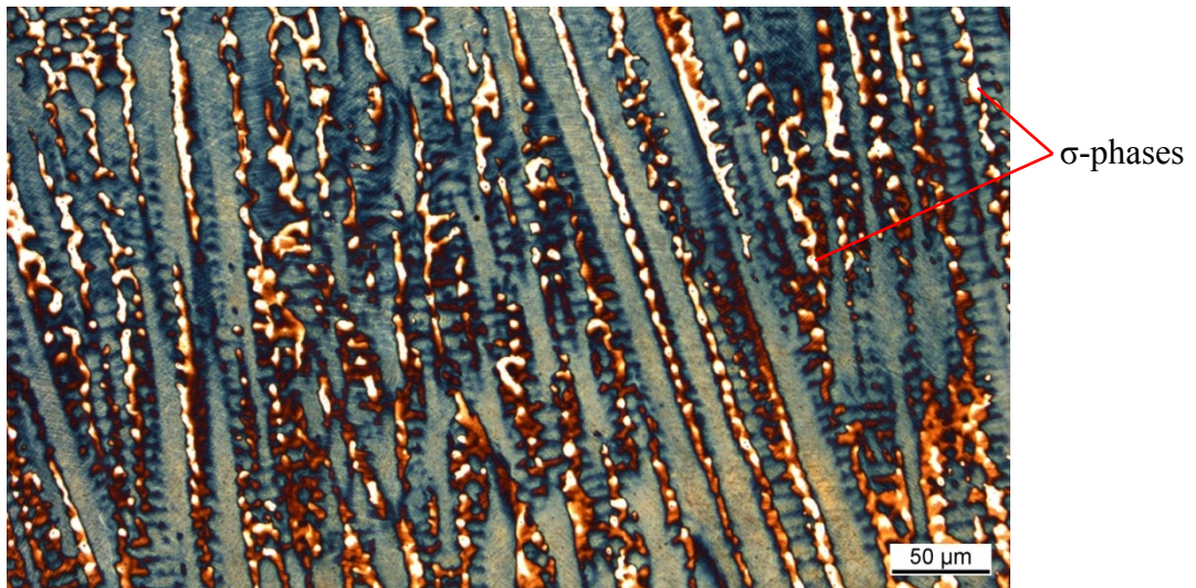
picture 19: Ultimet Alloy, 600°C, 60° angle of impingement, 200 x magnification, Beraha II
