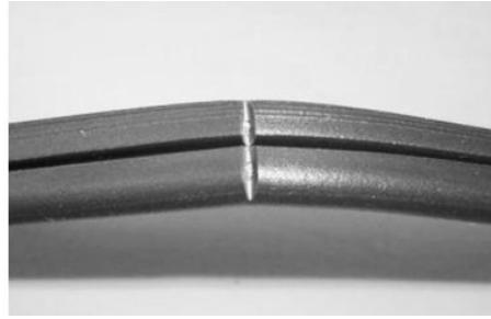
Figure 104: Damage done on a cable specimen (SPT2) for testing
