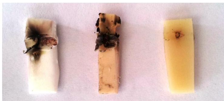
Figure 34: Effect on polymers of thermal stress from glowing Left: PUR / middle: PVC / right: halogen free polymer
