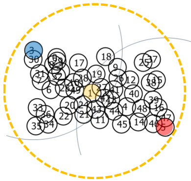
Figure 4-4: example of very high density scenario (the minimum number of hops between the two furthest nodes is 2 hops)
