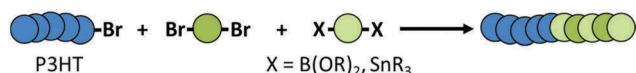
Scheme 16 Preparation of block copolymers utilizing AA/BB-type monomers for the second block in combination with P3HT as the first block.
